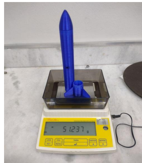
Fig. 4: Measuring the mass of model rocket 3D printed.
